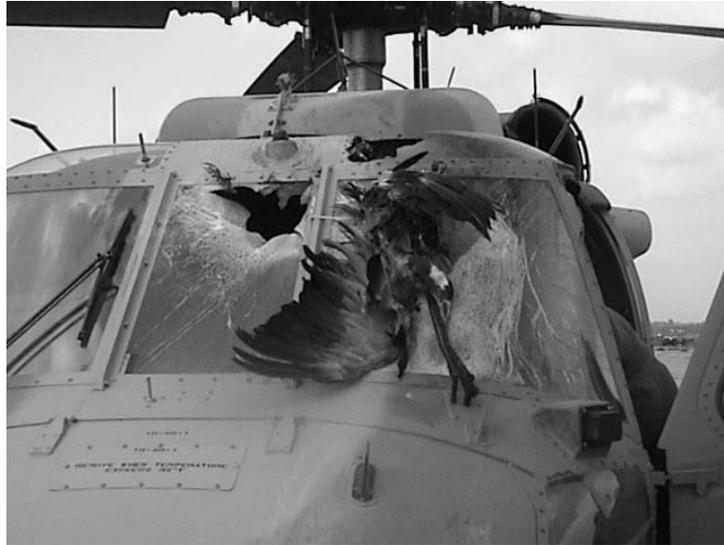
Fig. 1. Natural hazard - helicopter bird strike
